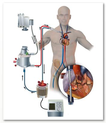
▶ Figure 1: ECMO involves the placement of a catheter in a central vein to draw blood through a chamber where CO2 is removed and oxygen infused into the blood cells. The blood is then pumped back into the body at either a vein (veno-venous, for pure pulmonary support) or an artery (if cardiac support is needed to maintain vital organ function).
